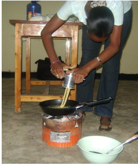
Figure 4 - Demonstrating Cold Extrusion of Bean Snack
